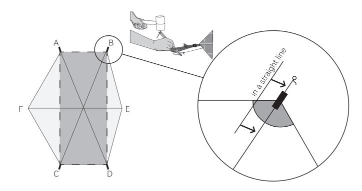
Step 1: Secure the four corner pegs (A, B, C, D) to form a perfect rectangle. (Do not install pegs E and F at this stage.)
